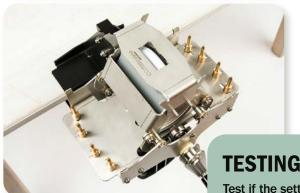
Test if the settings of the TURBO wrapper are correct by placing a mug in the mug support and then lift the lever as if you were going to wrap the mug. If the wrapper arms automatically fall down, then your TURBO wrapper is correctly set.
